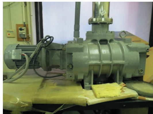
Figure 8. Photo of mechanical booster.
