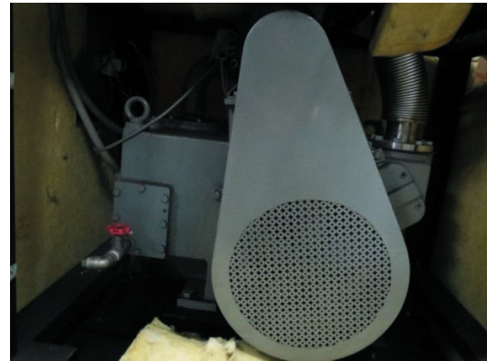
Figure 7. Photo of rotary pump.
