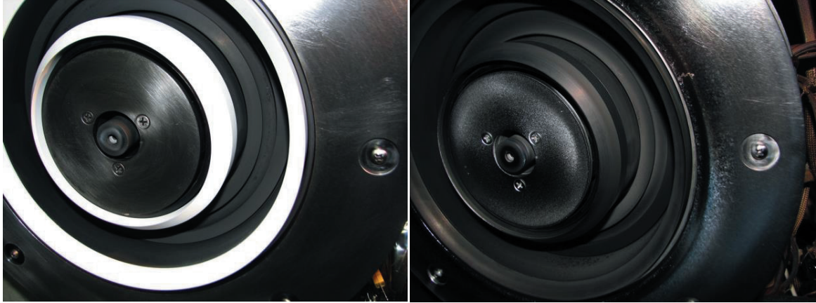
Fig. 1. Left: H6MS thruster before wear testing. The acceleration channel rings appear white and no surface roughening of the inner pole surface is evident. Right: The H6MS after a 150-h wear test in a JPL facility at 300 V and 20 A. The channel rings appear dark as the reduced erosion rates fell well below the deposition rates, allowing for build-up of carbon onto the ring surfaces. Roughening of the inner and outer pole surfaces became evident suggesting some sputtering could have occurred.
