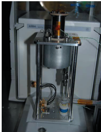
Fig. 4 Setup for calibration of the MOOG VPS03-002 Cold Gas Thruster on the Mettler Toledo AX 504 balance [7].
