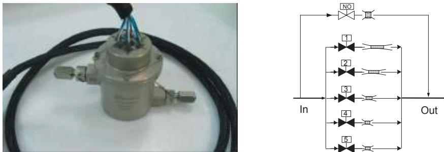
Figure 3 - Digital Xenon Flow Controller (DXFC): flight model (left) and block diagram (right)
