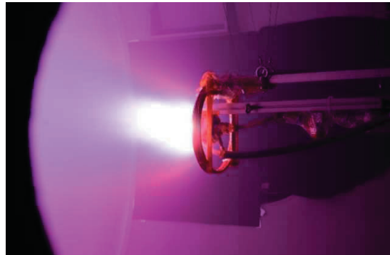
Figure 10. Time exposure photograph of interaction between the injected plasma and the magnetic field (Experimental result in case for the magnetic nozzle mode: solenoid coil + plasma injector).
