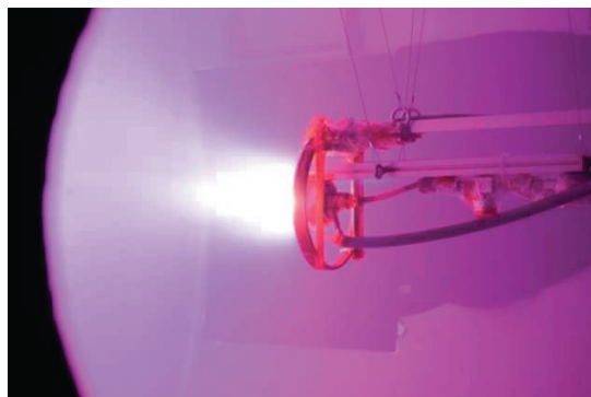
Figure 11. Time exposure photograph of interaction between the injected plasma and the magnetic field (Experimental result in case for the magneto plasma sail with magnetic nozzle mode:magnetic sail + magnetic nozzle).
