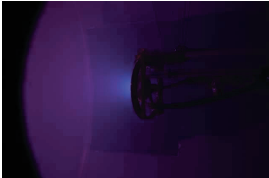
Figure 9. Time exposure photograph of interaction between the solar wind plasma and the magnetic field (Experimental result in case for the magnetic sail mode: solar wind simulator + solenoid coil).
