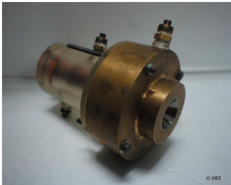
Figure 6. WEPS DC arc jet thruster (Photo) 7
