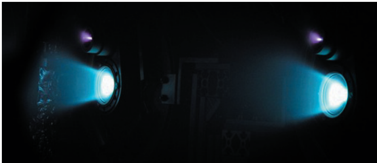
Figure 4.4. Parallel operation of two HEMP-Thrusters in dual-firing mode.
