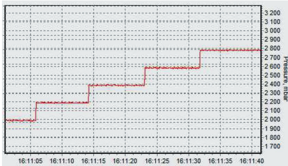
Figure 4. Pressure step up from 2.0 bar to 2.8 bar in 200 mbar steps (xenon).
