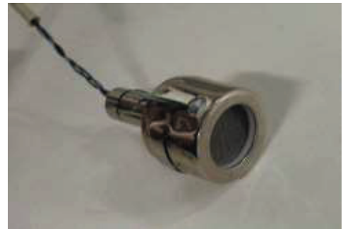
Figure 4. Energy Analyzer designed and produced at the UnBPPL.
