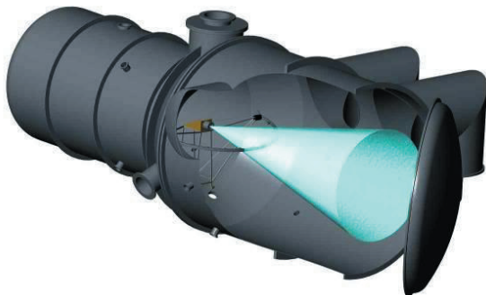
Figure 1. LEEP2 schematic showing location of thruster and typical T6 beam divergence angle
