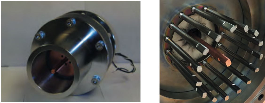
(a) Photograph of the SBT, not mounted to the CF flange. (b) Photograph of the M-SPG thruster, mounted to the CF flange.
