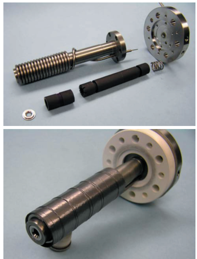
Fig. 4. The 1.5-cm dia. LaB 6 hollow cathode with 3-mm dia. heater installed (top) and heat shield installed without the keeper (bottom).
