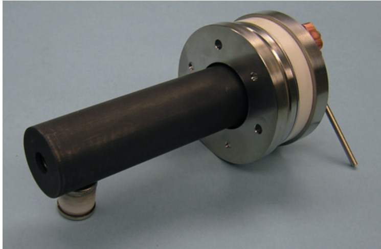
Figure 1. Second generation laboratory model lanthanum hexaboride hollow cathode.
