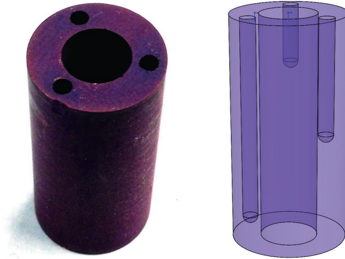
Figure 3. Photo and schematic of axial thermocouple wells in the lanthanum hexaboride insert.
