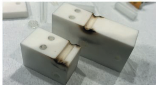
Figure.18 Cavity parts of the new PSF-PPT after 300 shots.
