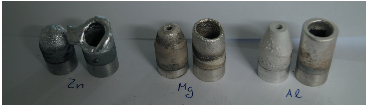
Figure 8. Photo of the eroded cathodes after the 6 experiment series. The total erosion times can be found on Table 1. Noteworthy is the meltdown of the zinc tube cathode.
