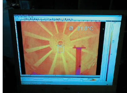
Figure 5. Infrared image of the water cooled beam dump target in vacuum.
