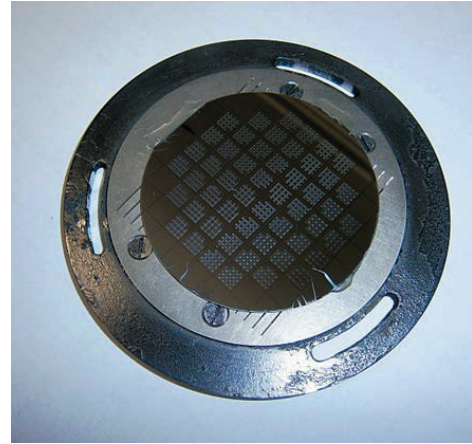
Figure 9. Sputter target based on a 2-inch wafer with regular pattern.
