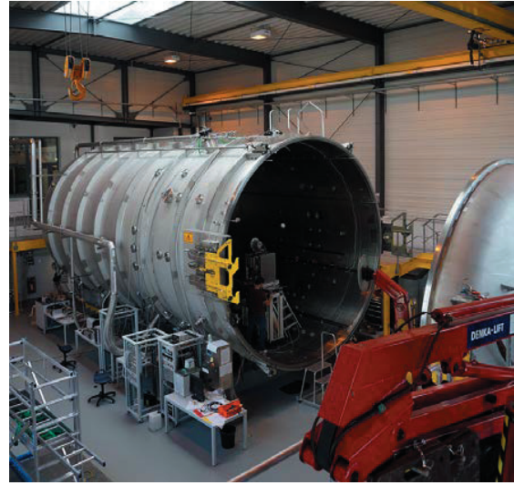
Figure 1. View into the open vacuum chamber of the STG-ET facility.
