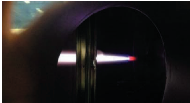
Figure 1. Sitael S.p.A. AT-1k arcjet firing in SPF Vacuum Facility in SPF
