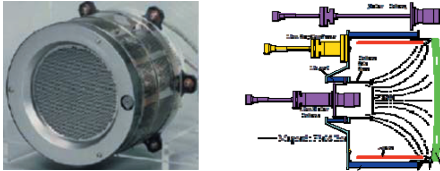
Figure 1. 20 mN class Ion Thruster and Configuration
