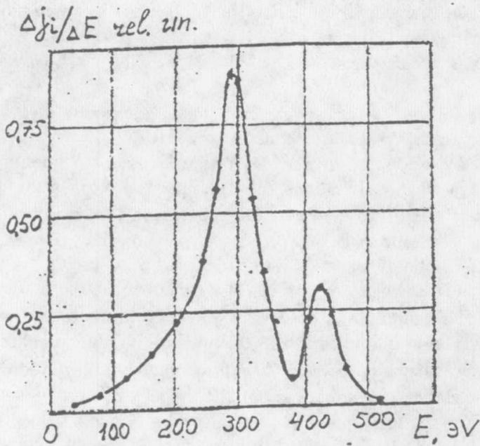
Fig.3. The ion flow energy spectrum.
