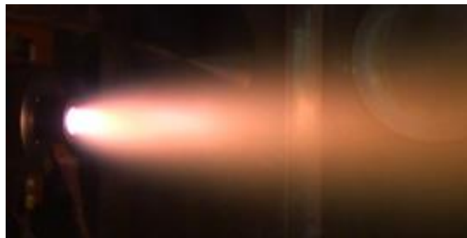
Figure 16. Photo of plasma plume of prototype anode-radiation-cooled arcjet thruster.
