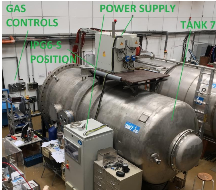
Fig. 4 IPG6-S refurbished facility
