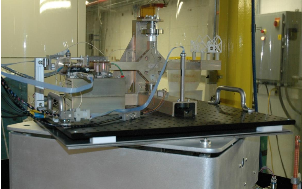
Figure 3. Torsional thrust balance mounted on vibration isolator.
