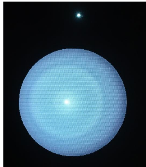
Figure 7. DEV-C thruster during stable operation. Photo taken in VF-16 at a beam current of 2.00A and beam voltage of 1179V. Photo taken by George Soulas.
