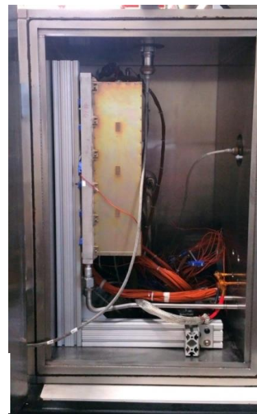
Figure 5. PPU installed for functional testing (above) and in TVAC chamber for temperature testing under vacuum (right).
