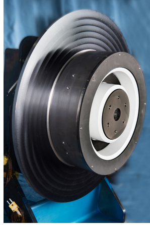
Figure 3 The 12.5 kW HERMeS Technology Development Unit 3 (TDU-3).
