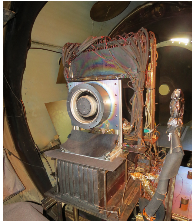
Figure 3: The H9 SN03 installed in the Owen's Chamber at the Jet Propulsion Laboratory for thrust measurement testing.
