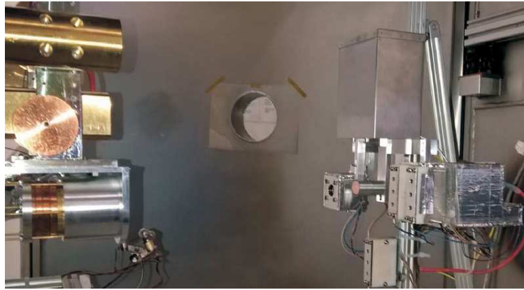
Figure 4. View into the test chamber: the swivel arm (on the right) equipped with the force probe, Faraday cups and a retarding-field analyzer in front of the HEMP thruster (on the left).
