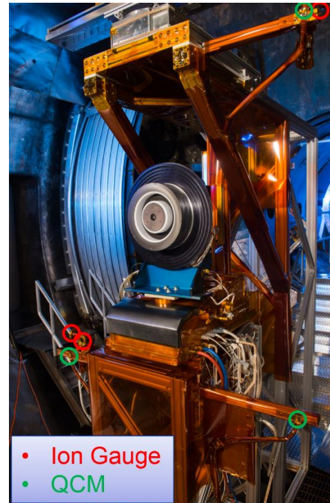
Figure 10. QCM and ion gauge location on the VF-6 test setup.
