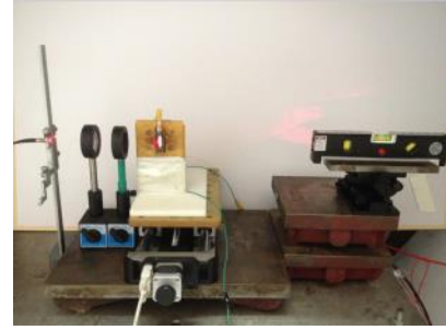
(b) Spectroscopic emission experiment system inside the vacuum chamber (positioning laser and calibration light source on the right)
