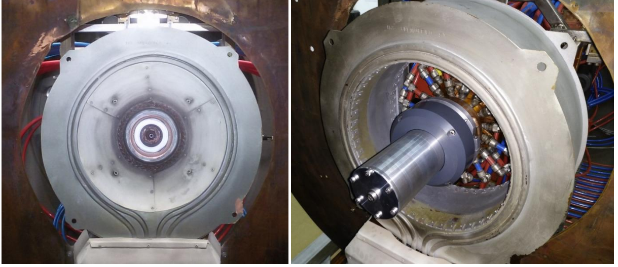
Figure 4. Mounted SX3 thruster and SX coil assembly (left) and implemented electrode interlink (150 mm) for short circuit measurements (left).
