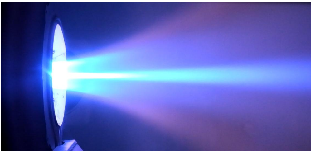
Figure 15. Visual plume appearance at 400 mT, 65.7 kW, 428 A, 12+48 mg/s argon (BN 3), (#067: 2.16 N, 3670 s, 56 %, 32.9 mN/kW, 1.083 kJ/mg).
