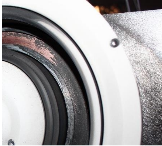
Figure 9. Post-test Inspection of the HT5k LL ceramic.
