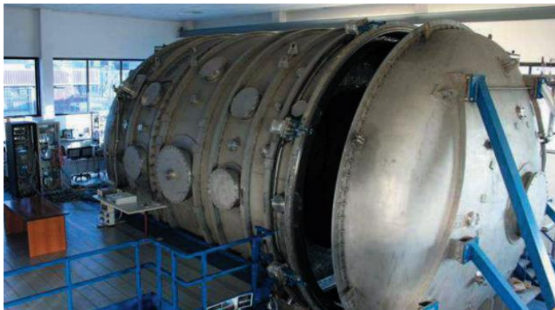
Figure 3. SITAEL's IV10 vacuum test facility
