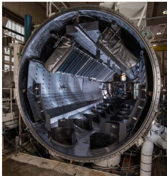
Figure 2. TDU-3 installed in NASA GRC VF-5.
