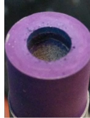
(b) Detail of the contaminant deposited on the inside of the insert.
