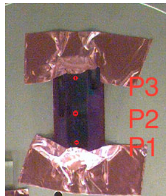
(b) Insert piece inside the KRATOS Ultra XPS at Caltech
