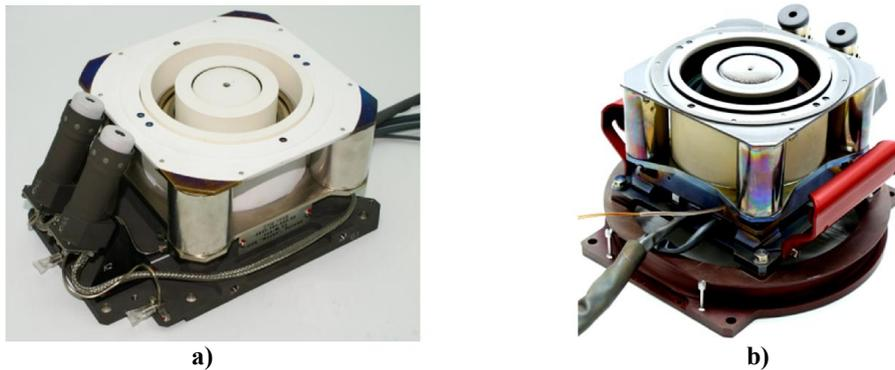
Figure 1. General views of the SPT-100D (a) and SPT-100BM (b) thruster.
