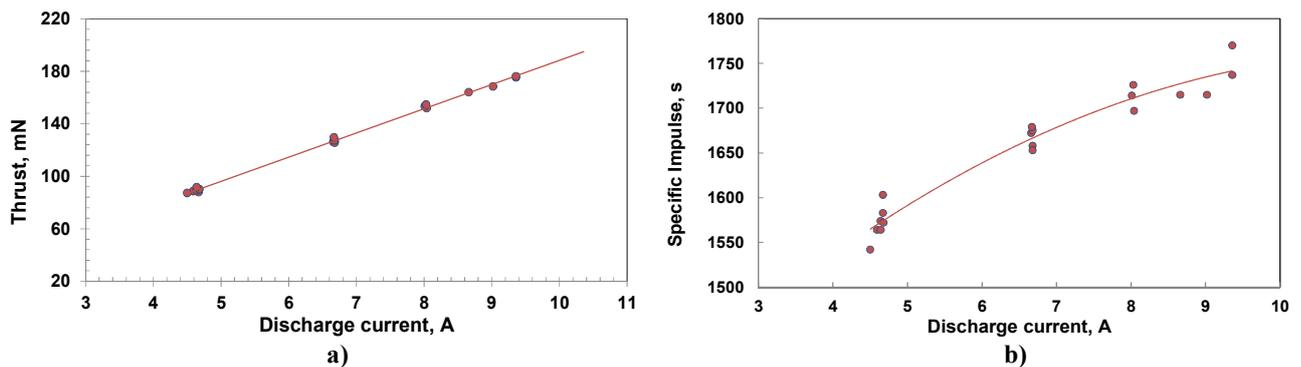
Figure 5. SPT-100D thrust (a) and specific impulse (b) at discharge voltage  $U_d = 300$  V.
