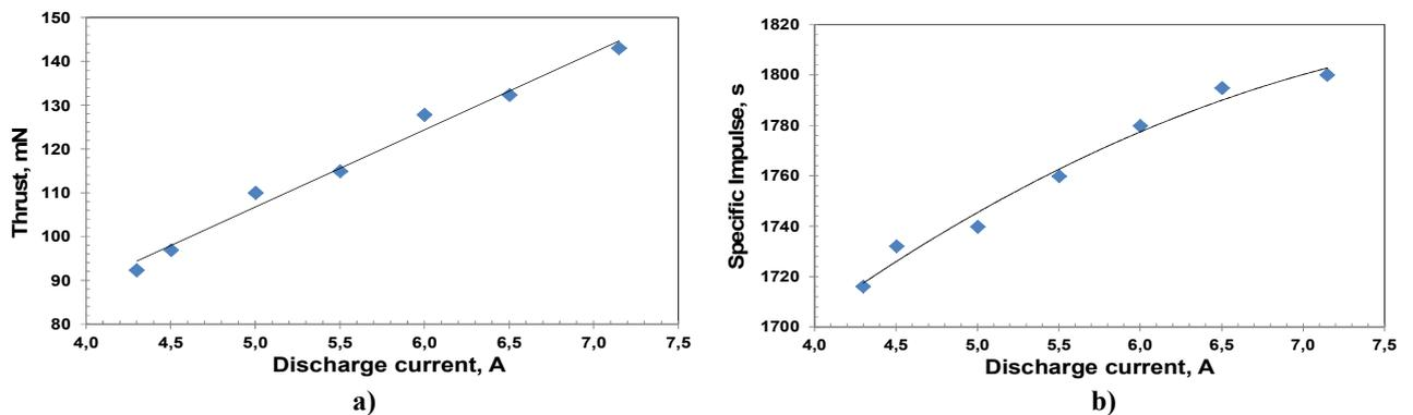
Figure 6. SPT-100D thrust (a) and specific impulse (b) at discharge voltage  $U_d = 350$  V.
