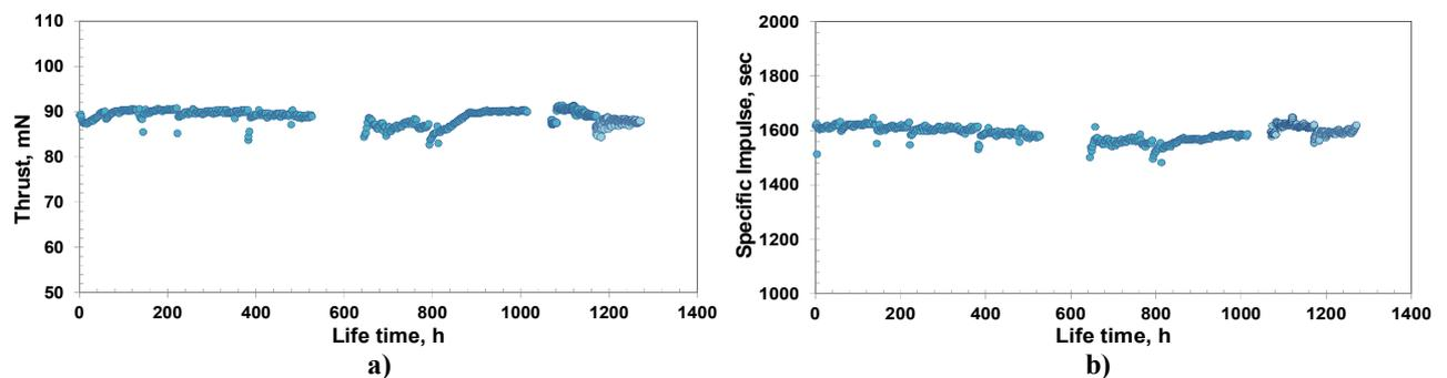
**Figure 9. SPT-100BM thrust (a) and specific impulse (b) during the life time test.**
