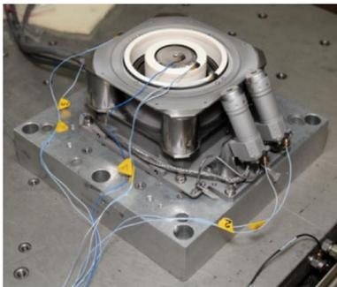
Figure 2. SPT-100D mounted on the vibration plate.
