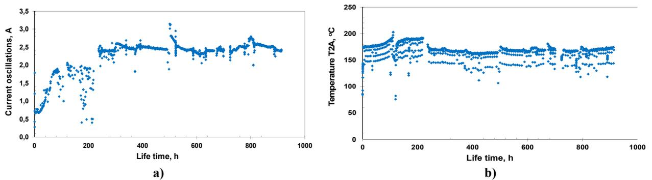
**Figure 8. SPT-100D discharge current oscillations (a) and thruster temperature in the reference point T2A (b).**
