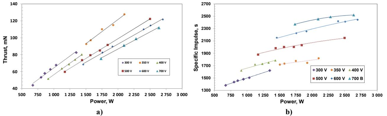
Figure 4. SPT-100D performance test results: Thrust - Power diagram (a). Specific impulse - Power diagram (b).
