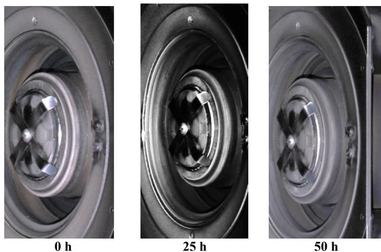
**Figure 6. SPT-100D operation in the estimated end of the thruster life time. Erosion is practically absent.**
