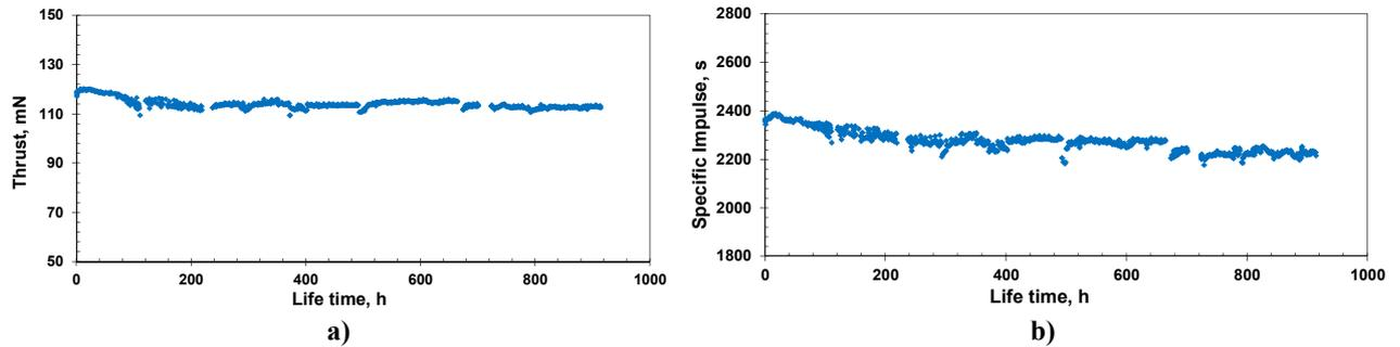
**Figure 7. SPT-100D thrust (a) and specific impulse (b) in the process of long-term operation.**
