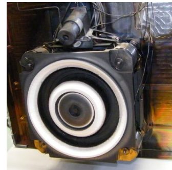
Figure 8. PPS®5000 EQM1 after 1,700 hours of operation at 5 kW of discharge power.
