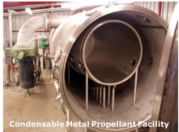
Figure 9. Vacuum chamber for testing electric thrusters with condensable-metal propellants, including lithium. The vacuum chamber is 3-m dia. by 8-m long. The water-cooled liner is 5.16-m long with a pumping surface area of 38 m 2 resulting in a lithium pumping speed of 9,000,000 L/s.
