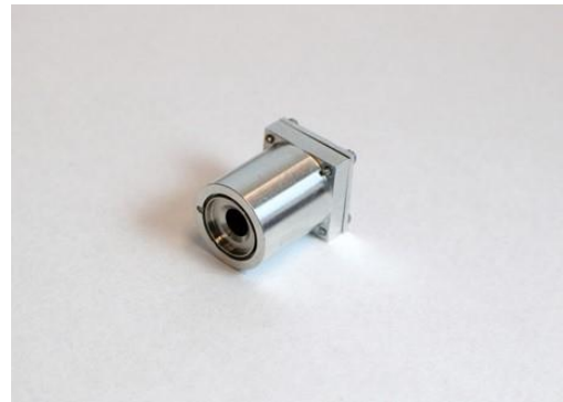
Figure 2. Highly miniaturized NanoFEEP thruster, dimensions: diameter 13 mm, length 21 mm
