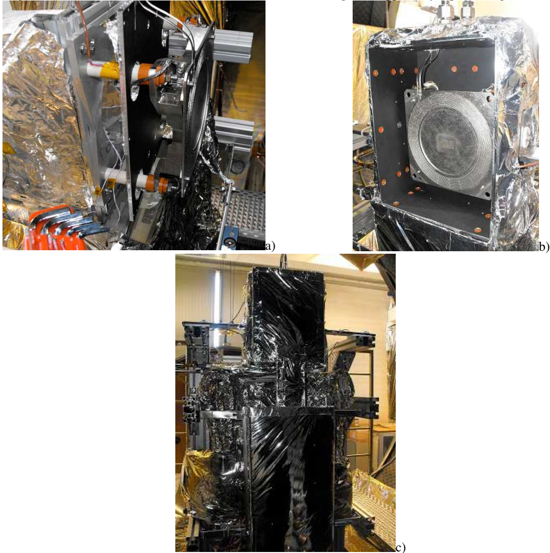
Figure 4. Installation of the mock-up plate and the thermal shroud on the thrust balance.
