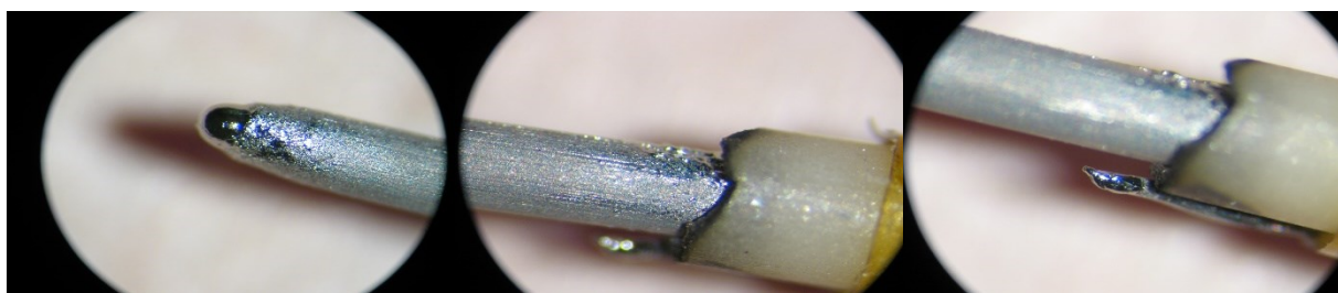
Figure III-9: Tungsten cathode after testing breadboard version 4. Left, molten tip. Center, molten/worn cathode close to the PTFE surface. Right, molten ignition wire (tungsten).
