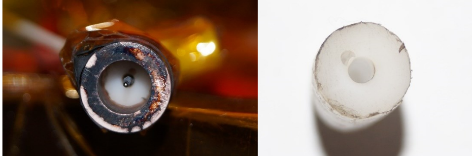
Figure III-10: Left, breadboard version 4 after 2072 pulses showing deposit at the anode's front. Right, showing the PTFE surface after 2072 pulses.
