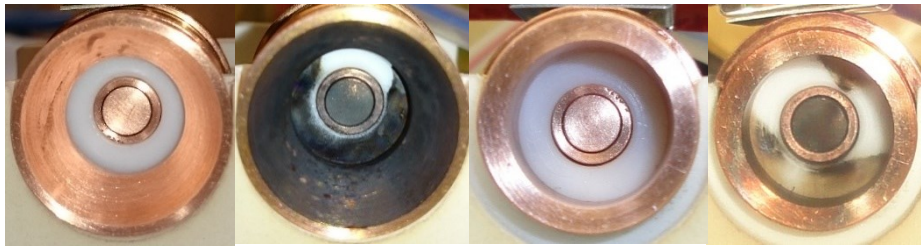
Figure II-2: From left to right. Convergent/divergent nozzle as anode before the test. Convergent/divergent nozzle after 5600 pulses. Cylindrical anode before the test. Cylindrical anode after 5600 pulses.
