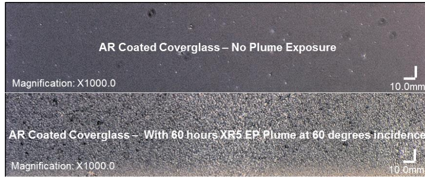
Figure 16. Magnified BOL & EOL Coverglass Images. Pristine AR Coated Coverglass (top) compared to a coverglass with the AR coating removed and textured by the EP plume (bottom).
