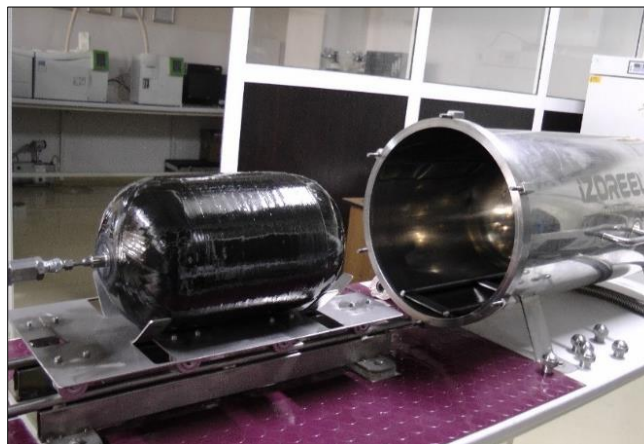
Figure 7. Helium Leakage Test Setup
