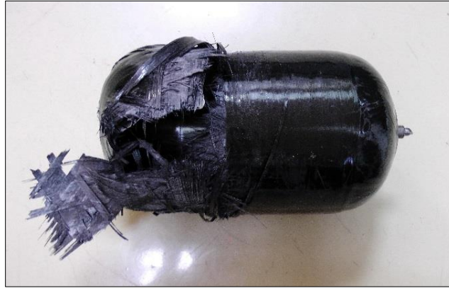
Figure 8. Failure of XPT after Burst Test
