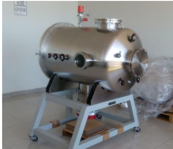
Figure 13. The ASP Lab new vacuum chamber, with a 2000 l/s turbomolecular pump mounted below it. Preliminary to experimental work, which will include thrust measurements, carried out with a torsional balance similar to that developed at LCP/INPE 14 , theoretical investigations have characterized PPT performance through extensive analysis of experimental data available in the literature, yielding new semi-empirical relations extremely useful for initial thruster design. This was especially needed for the low-power operating regime, where existing relations did not accurately describe PPT behavior for all discharge configurations, 7 and allowed some interesting insight into preliminary thruster design. 16
