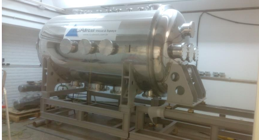
Figure 12. The new 1.5-m diameter vacuum facility at the Plasma Laboratory (LP), IF/UnB. to a high vacuum by using turbomolecular pumps. A direct thrust measurement system is being developed and will be installed in this new chamber.
