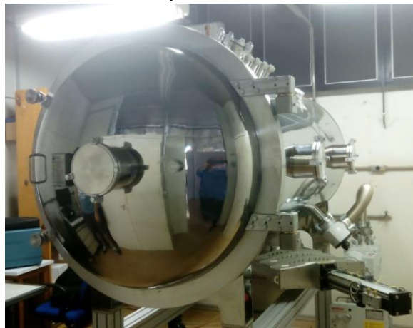
Figure 10. The new 1-m diameter vacuum facility at LCP/INPE.
