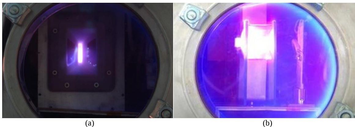
Figure 8. DD-PPT X1 (a) and DD-PPT X2 (b) being tested.
