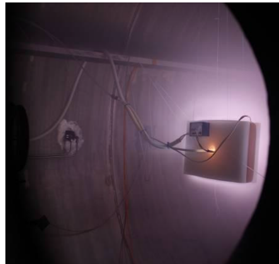
Figure 4. 6U-scale magnetoshell operating in vacuum using Argon at 200 sccm, 300 W RF power, and 172 G field. 7
