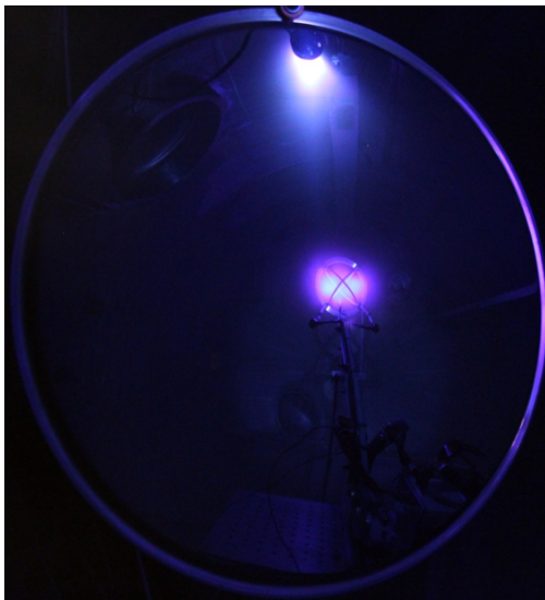
Figure 3. Demonstration of drag on a magnetoshell in vacuum. 1
