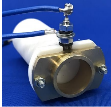
Figure 21. The single discharge room PPT.
