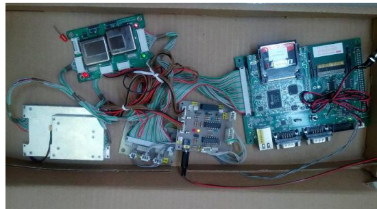
Figure 12. Ground experiment on malfunction of satellite.
