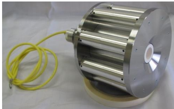
Figure 25. Photo of the cylindrical-type Hall thruster.
