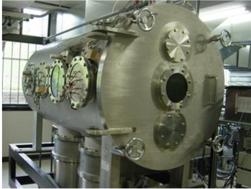
Figure 5. Vacuum chamber and pumping system.
