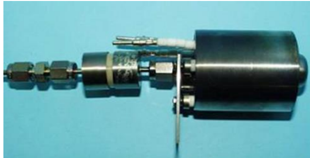
Figure 8. Photo of the hollow cathode.
