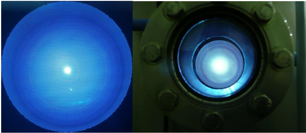
Figure III-1 RCDC MSL1 in operation with xenon at Mars Space Ltd propulsion laboratory
