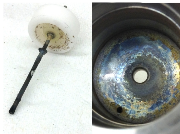
(b) Surface deposition on anode (left) and cathode (right) in PKR-251 cold cathode vacuum meter.
