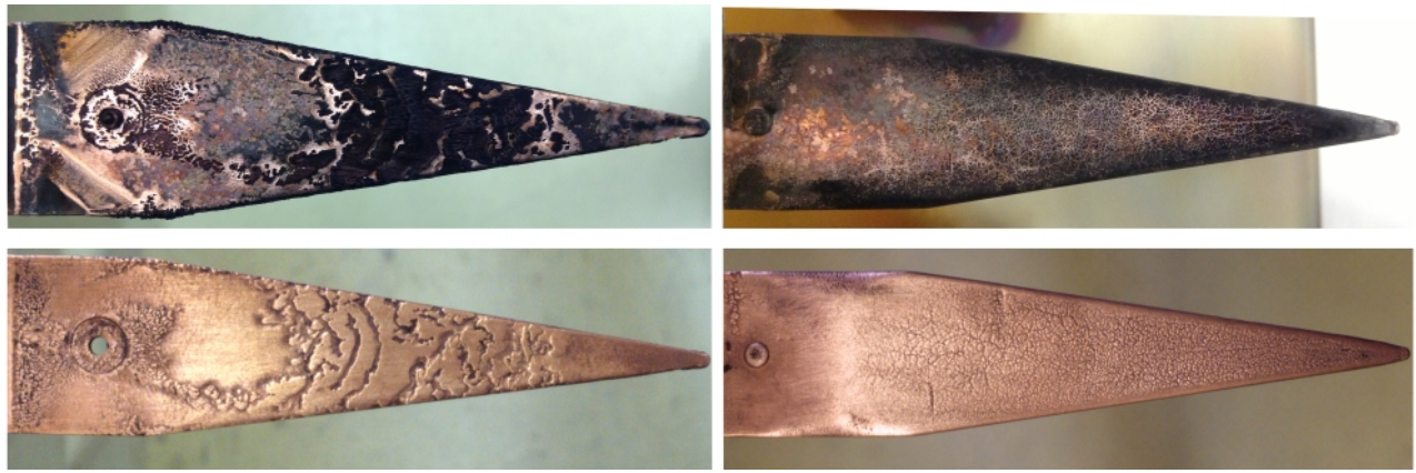
Figure 5. Cathode (left) and anode (right) depositions (top) and erosion (bottom) at the end of testing (EOT).
