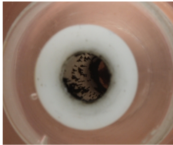
(b) Carbon dome deposition growth after 11000 pulses for transition to full carpet layer coverage.
