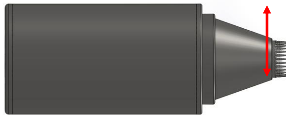
Figure 2 Orientation of propellant tank during testing in a terrestrial laboratory. The red arrow indicates the maximum contribution to hydrostatic pressure at the bottom of the crown when the tank is filled. In order to keep this pressure low, the tank is long and uses a small diameter.
