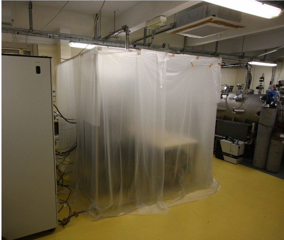
Fig. 2 Thermal shield installed in order to serve as a low-pass filter for the temperature variations of the room due to the pulsed air conditioning system.
