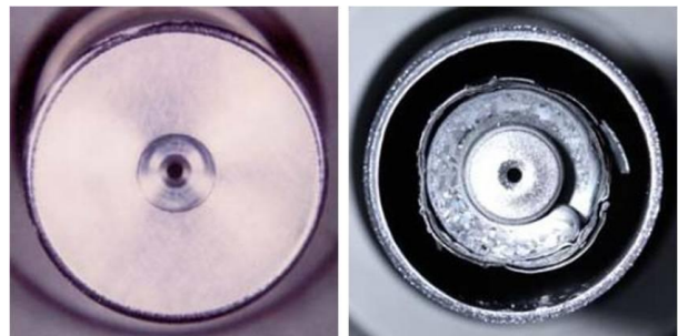
Figure 13. NSTAR ELT discharge cathode assembly front view at BOL (left) and after 30,352 h (right).
