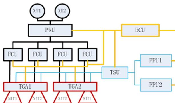
Figure.5 the IEPS for GEO Satellite NSSK
