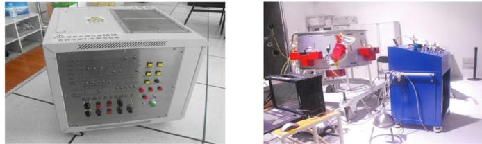
Figure 11 LIPS-200 TI and XFE developed for SJ-9A IEPS
